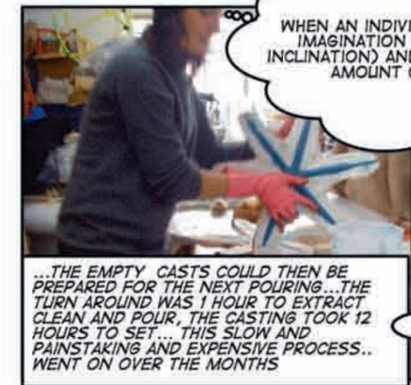
...THE EMPTY CASTS COULD THEN BE PREPARED FOR THE NEXT POURING...THE TURN AROUND WAS 1 HOUR TO EXTRACT CLEAN AND POUR, THE CASTING TOOK 12 HOURS TO SET... THIS SLOW AND PAINSTAKING AND EXPENSIVE PROCESS... WENT ON OVER THE MONTHS
